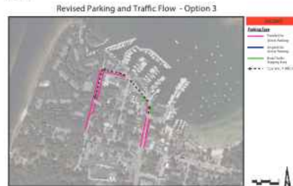
Figure 24. Option #3 - Consider creating one way loop from intersection of Spruce Street and Maple Street with traffic flowing counter clockwise to the intersection of Cottage Row and Maple Street. Re-stripe parallel parking along Cottage Road and add parallel parking along south side of Spruce Street by the Alibi. This option would add approximately twenty-five (25) parking stalls. Convert portion of existing stalls near west launch to a staging and maneuvering area for boats.
